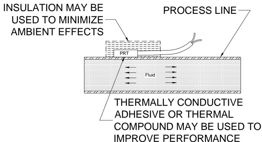
**FIGURE 1 – TYPICAL SURFACE SENSOR INSTALLATION**
