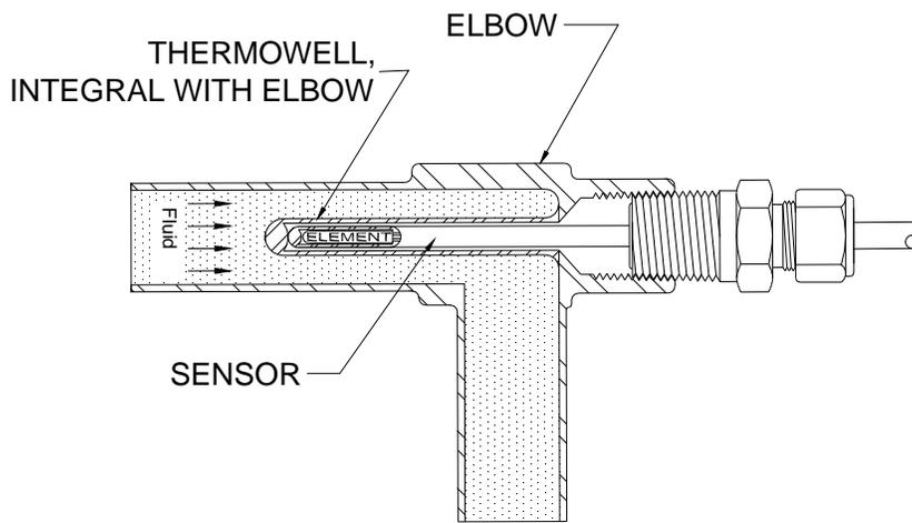
**FIGURE 4 – INDIRECT IMMERSION SENSOR INSTALLATION**
