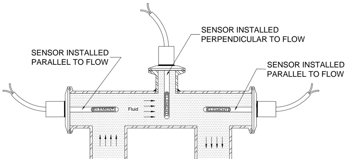
**FIGURE 3 – DIRECT IMMERSION SENSOR INSTALLATIONS**
