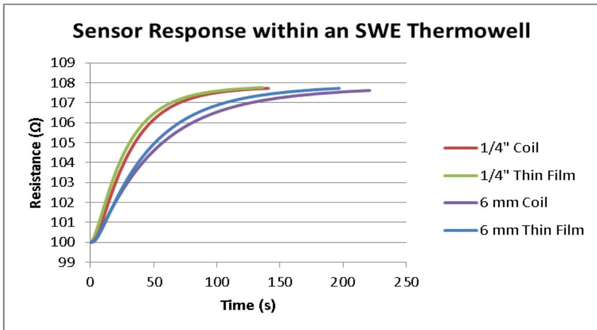
Figure 2: Sample Time Response Curve for Each Construction with an SWE Thermowell
