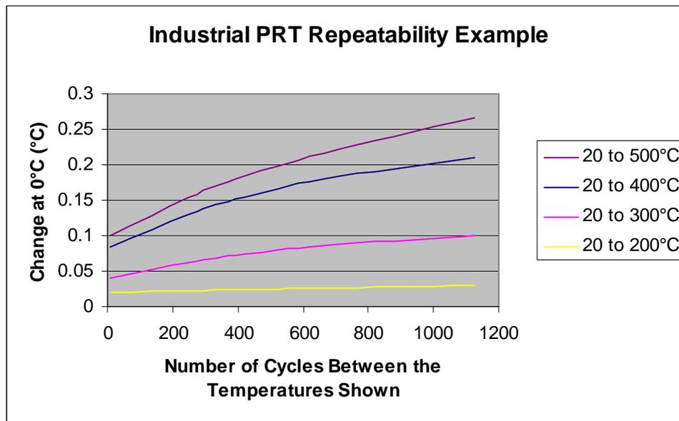
By examining the figure there are several generalizations that can be made about repeatability. The generalizations listed below hold true for the behavior of most industrial PRTs, however the actual values, maximum temperature ranges, etc., will all be unique based on the specific PRT design. If a better understanding is needed regarding a specific PRT, the manufacturer of that PRT should be consulted.
