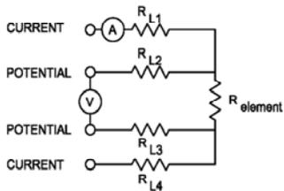
$$R_{\text{measured}} = \frac{V}{A}$$
