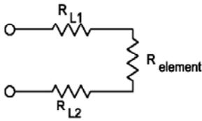
$$R_{\text{measured}} = R_{L1} + R_{\text{element}} + R_{L2}$$
