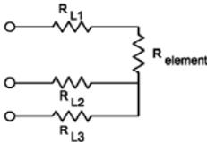
$$\begin{aligned} R_{\text{measured}} &= R_{L1} + R_{\text{element}} + R_{L2} - [R_{L2} + R_{L3}] \\ &= R_{L1} + R_{\text{element}} - R_{L3} \\ &= R_{\text{element}} \quad (\text{if } R_{L1} = R_{L3}) \end{aligned}$$
