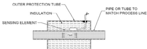
Another solution is to mount a sensor on the pipe surface. This approach however can compromise accuracy.
