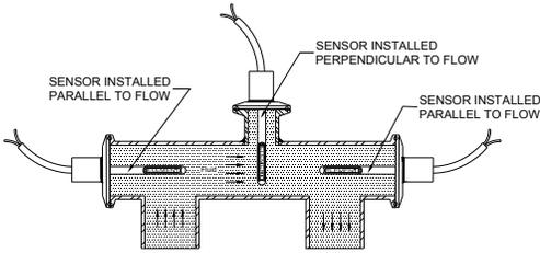
Installation into a tee with the sensor parallel to the flow can allow for longer immersion length.
