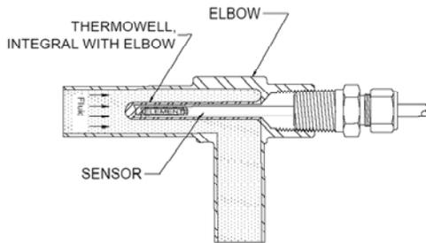
A special elbow fitting with an integral thermowell allows for sufficient immersion length in tubes down to 0.5" diameter.
