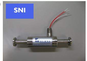
We modified the SNI design to mount on the surface of the existing tubing by creating a half-shell design. This half-shell left tabs on the sides that could be used to hose clamp the unit in place. Hose clamps created an easy way to install the sensor on the tubing while providing the component integrity required. No welding was needed for installation.
